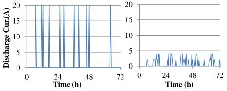
The discharging current with distributed design (left) vs. ours (right)
