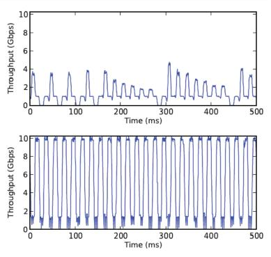
Bandwidth seen by the receiver (top) in case of regular TCP adapting to changing link capacities, and (bottom) when the TCP flow is controlled by TDMA.
