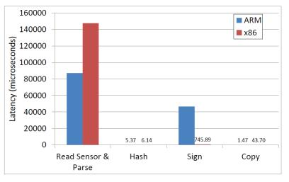
Latency breakdown on ARM and x86 platforms shows the latency of reading and parsing the sensor output, then hashing, signing and copying the results.
