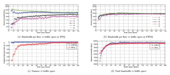
$\label{eq:comparison} \mbox{ Comparison between Weighted Fair Queuing (WFQ) and Enhanced WFQ (EWFQ) on fairness and attained bandwidth with respect to buffer space$
