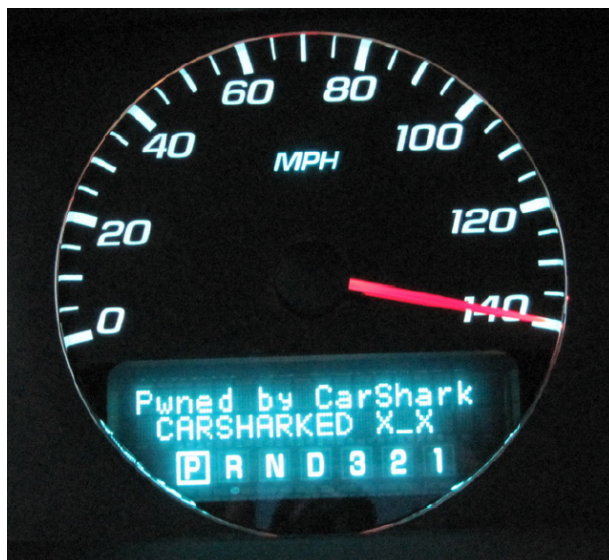
Arbitrary message and false speedometer reading visible on the driver information center; note that the speed is at 140mph even though the car is in Park.
