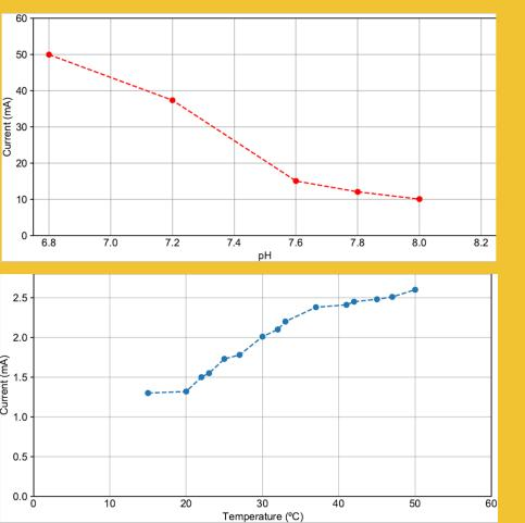
Corrosion current decreases with the increase in pH of the electrolyte
