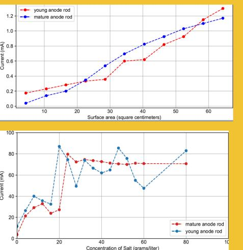
Corrosion current is directly proportional to the surface area in contact with the electrolyte
